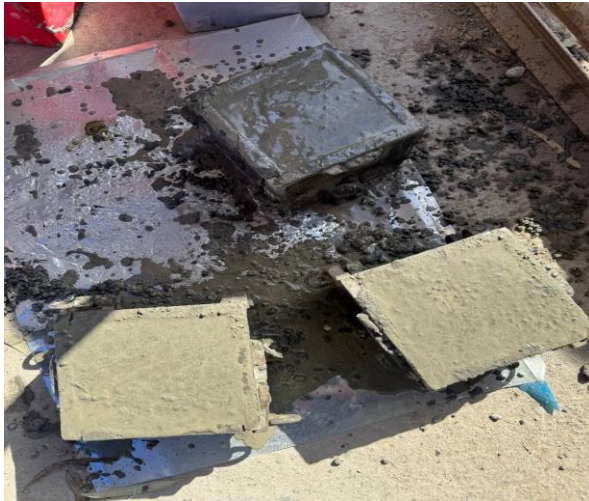
Figure 3: Pouring fresh concrete into molds after compaction on the vibrating table
