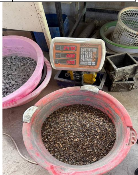
Figure 2: Weighing of coarse aggregate (gravel) using the INGCO digital scale
