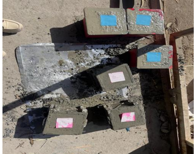
Figure 4: Concrete specimens after casting with identification labels for the control and modified mixes
