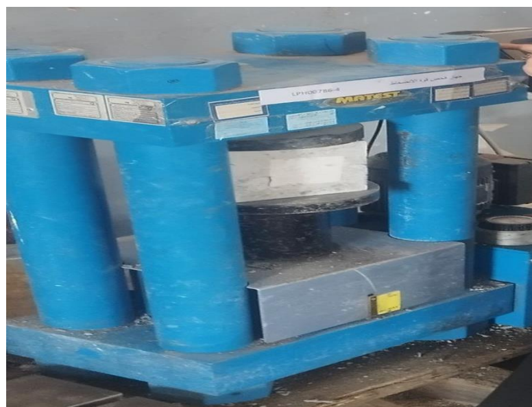
Figure 5: Compressive strength testing of concrete specimens using the MATEST compression testing machine (LPH00786-4)
