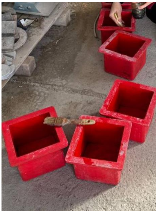
Figure 1: Cube molds (150×150×150 mm) after oiling in preparation for casting
